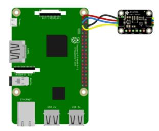
Pi 3V to sensor VCC (red wire)
