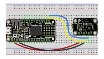
Board 3V to sensor VIN (red wire)
