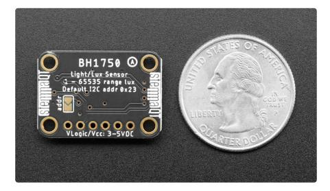
The BH1750 provides 16-bit light measurements in lux, the SI unit for measuring light making it easy to compare against other values like references and measurements
