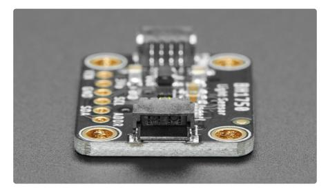
To make things easier and a bit more flexible, we've also included <u>SparkFun Qwiic</u> () compatible <u>STEMMA QT</u> () connectors for the I2C bus so you don't even need to
