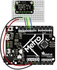
Connect Vin to the power supply, 3V or 5V is fine. Use the same voltage that the microcontroller logic is based off of. For most Arduinos, that is 5V Connect GND to common power/data ground
