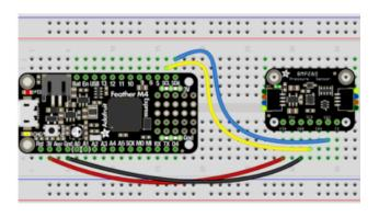
Board 3V to sensor VIN (red wire on STEMMA version) Board GND to sensor GND (black wire on
