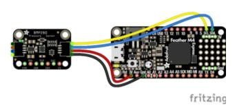
And an example of a Feather M0 wired with hardware SPI:
