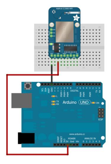
Next, connect the enable and interrupt lines: VBEN to Digital 5 IRQ to Digital 3
