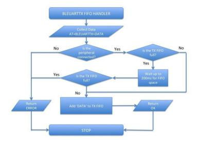
Note: The TX FIFO full check will happen for each GATT transaction (of up to 20 bytes of data each), so large data transfers may have multiple 200ms wait states.
