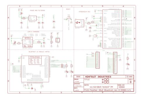
We've changed the regulator from an SPX3819 to AP2112 - it has lower dropout but cannot handle higher than 6V
