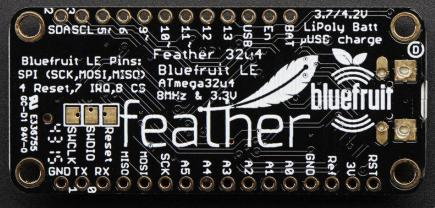
The DFU pin is accidentally labeled GND on the bottom, sorry about that! it should be labeled DFU, dont use it as a GND
