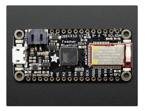
At the Feather 32u4's heart is at ATmega32u4 clocked at 8 MHz and at 3.3V logic, a chip setup we've had tons of experience with as <u>it's the same as the Flora</u> (). This chip has 32K of flash and 2K of RAM, with built in USB so not only does it have a USB-to-Serial program & debug capability built in with no need for an FTDI-like chip, it can also act like a mouse, keyboard, USB MIDI device, etc.
