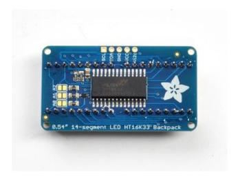
Check your work, making sure each pin is nicely soldered, and there's no cold solder joints or shorted pins
