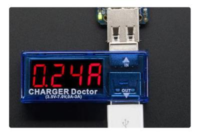
If you want to check the exact current draw during charge, try out a Charger Doctor between the USB port and charger. ()
