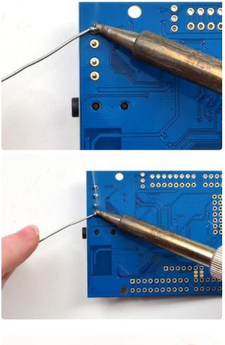
Solder the four pins with plenty of solder
