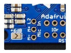
We break out the microphone/line in inputs, for recording audio. Some basic analog filtering is required depending on the electret microphone or amplifier. Check the VS1053 datasheet for how to connect up a mic!
