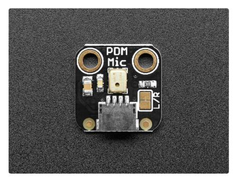
The 4-pin JST connector has 3V, GND, DAT, CLK connections that <u>can be used with</u> one of our JST-SH cables to make a flexible mic arrangement (). If you want a version with breakout headers, we have a version here (). An on-board solder jumper lets you change the mic from Left to Right channel
