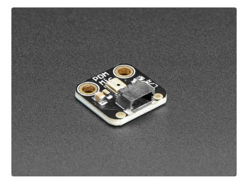
The first thing to note is that this sensor does not provide an 'analog' output like many of our electret microphone assemblies. So it's great for chips that do not have analog
