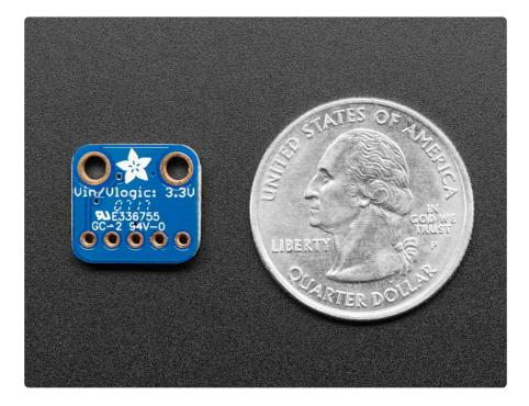
PDM is a little like 1-bit PWM. You clock the mic with a 1 MHz - 3 MHz clock rate, and on the data line you'll get a square wave out that syncs with the clock. The data line with be 0 or 1 logic output, with the square wave creating a density that when averaged will result in the analog value out.
