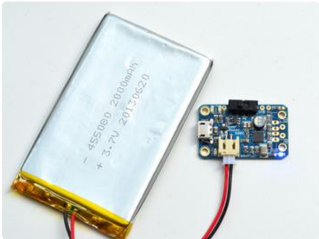
When the switch is to the left, the 5V power will be on, you can tell because the blue LED is lit
