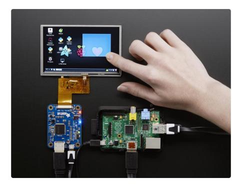
Its a mini HDMI decoder board! So small and simple, you can use this board as an all-in-one display driver for TTL displays, or perhaps decoding HDMI/DVI video for some other project. This breakout features the TFP401 for decoding video, and for the touch version, an AR1100 USB resistive touch screen driver.
