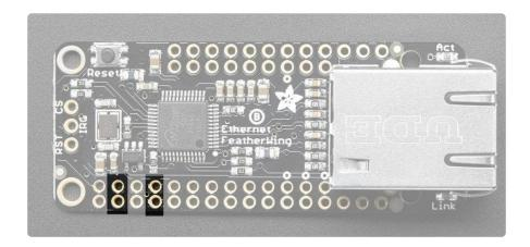
The WIZ5500 Ethernet chip (and really any ethernet chip) are fairly high current devices, requring about 150mA whether or not actively transmitting. The chip is powered from the 3.3V and GND pins indicated and does not have an internal regulator.
