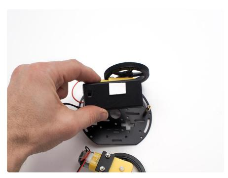
Cut a small strip of double stick tape and press it onto the side of the battery box with the 9V switch.
