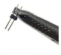
For this next step, you will need a set of pliers. First, grab the long header pins that are attached together and break them into 2 sets of 2 header pins. Then, grab them in the pliers like shown here, and then slightly bend them so they look like the next picture.
