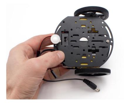
Place the battery box back in between the motors and stick it to the chassis
