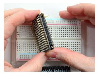
The LEDs face out and connect to the two side header strips.
