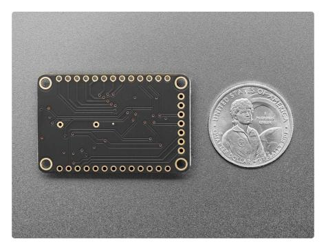
The IS31FL3731 is a nice little chip - it can use 2.7-5.5V power and logic so it's flexible for use with any microcontroller. You can set the address so up to 4 matrices can
