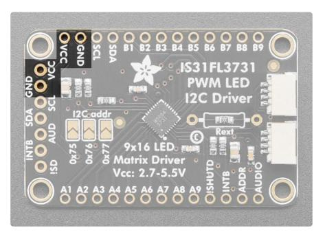
You can power the IS31 from 2.7-5.5VDC, but note that the same voltage is used for both power and logic.
