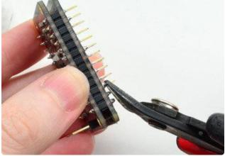
Now you can trim the long header with diagonal cutters. Cut one or two pins at a time
