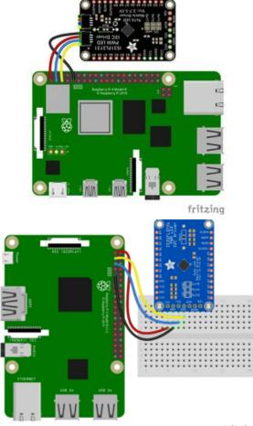
Pi 3V3 to breakout VIN Pi GND to breakout GND Pi SCL to breakout SCL Pi SDA to breakout SDA
