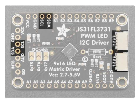
This chip uses I2C for control, it does not use clock stretching or repeated start. There are built in 20K pullups to VCC. You can run it as fast as 400KHz clock speed, but you may need to add additional 2K pullups from SDA and SCL up to VCC for higher speeds
