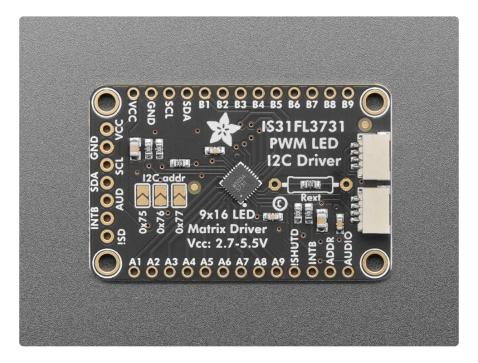
This chip is great for making small LED displays, and we even designed the breakout to match up with our ready-to-go LED grids in red, yellow, green, blue and white. Sandwich the driver and matrix breakout, solder together for a compact setup. Or you can DIY your own setup, just follow the LED grid schematic in the IS31FL3731 datasheet.
