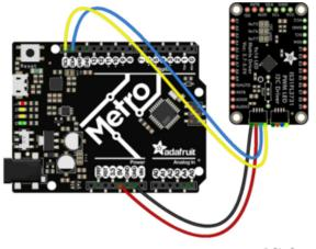
Board 5V to breakout VIN Board GND to breakout GND Board SCL to breakout SCL Board SDA to breakout SDA
