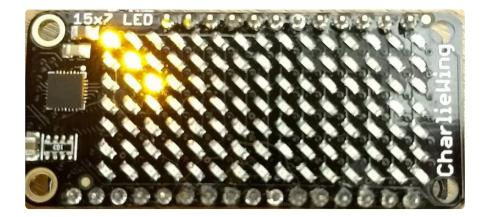
Notice how the first call switches to make frame 1 the active frame but doesn't display it because show is set to false. Then the frame pixel data is changed with fill and pixel
