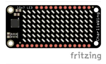
Assemble the CharlieWing by soldering headers onto the board. Once assembled, plug it into a Feather!
