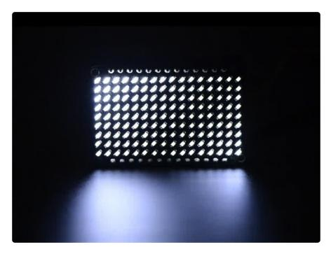
Pick up a driver board and your favorite color LEDs to match. You'll need to do some basic soldering to attach the driver backpack and matrix together, and run wires to your microcontroller, but its not too hard. Then install our Arduino or CircuitPython libraries to get some LEDs blinking immediately. Our library is Adafruit\_GFX compatible so you can draw lines, circles, text, and small bitmaps if you want more graphics control.
