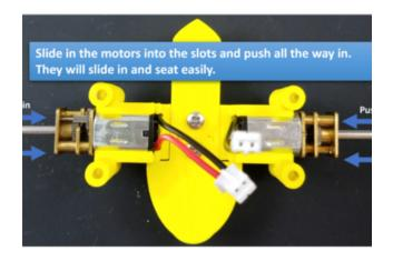
Slide in the 2 motors into the motor slots. They will slide in easily. There is no specific orientation for the motors.
