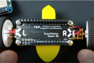
Install the wheels onto the motors. The wheels just press-fit onto the motor shaft. Ensure the flat surfaces on the motor and wheel line up and press.
