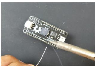
Place and solder the headers on the Robot board.
