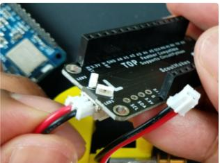
Connect the motor wires to the robot board. Notice the orientation of the root board with the TOP facing up.
