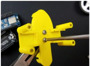
Insert the provided 2 screws (long) into the holes and tighten the nuts on the underside of the chassis. You will need a phillips head screw driver and a pair of pliers to hold the nut while its tightened.
