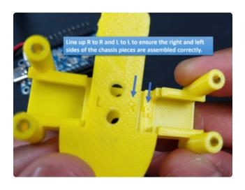
Assemble the robot chassis by bringing together the 2 plastic pieces. Ensure the sides line up as in the image below.
