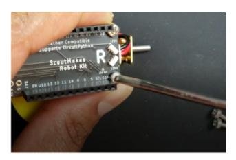
Screw in the robot board to the chassis using the 4 short screws provided.
