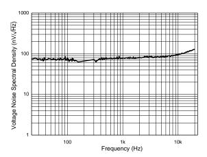
Figure 2. Input Voltage Noise in Zero-Drift Amplifier (AS2333Q)
