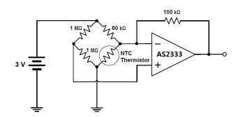
Figure 9. Bridge Circuit Amplification
