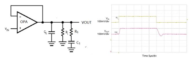
Figure 6. Circuit with Snubber Circuit
