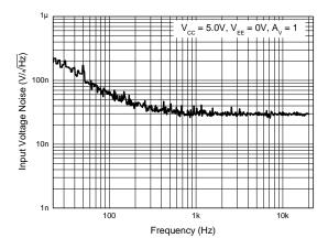
Figure 1. Input Voltage Noise in Conventional Amplifier
