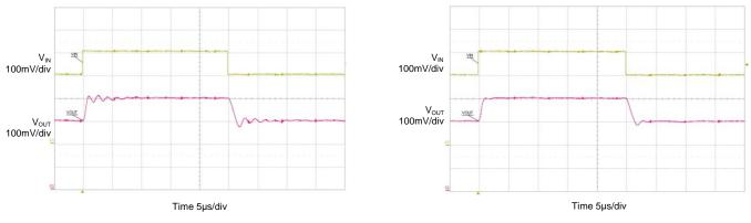
Figure 4. Test Result Without R<sub>NULL</sub>
