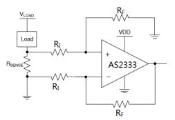
Figure 8. Low-Side Current Monitor Application
