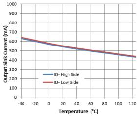
Figure 19. Output Sink Current vs. Temperature
