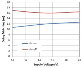
Figure 14. Delay Matching vs. Supply Voltage
