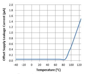
Figure 27. Offset Supply Leakage Current vs. Temperature
