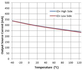
Figure 17. Output Source Current vs. Temperature
