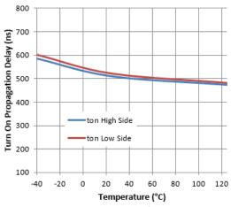
Figure 5. Turn-on Propagation Delay vs. Temperature
