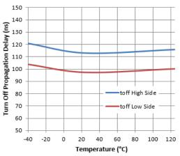
Figure 7. Turn-off Propagation Delay vs. Temperature
