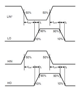
Figure 2. Switching Time Waveform Definitions
