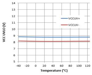
Figure 26. VCC UVLO vs. Temperature
