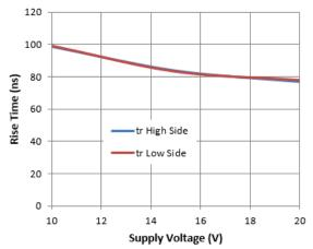
Figure 8. Rise Time vs. Supply Voltage
