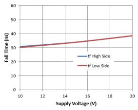
Figure 10. Fall Time vs. Supply Voltage
