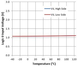
Figure 23. Logic 0 Input Voltage vs. Temperature
