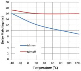
Figure 15. Delay Matching vs. Temperature
