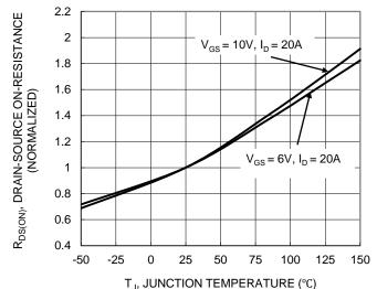
Figure 6. On-Resistance Variation with Temperature
