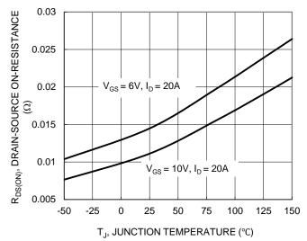
Figure 7. On-Resistance Variation with Temperature
