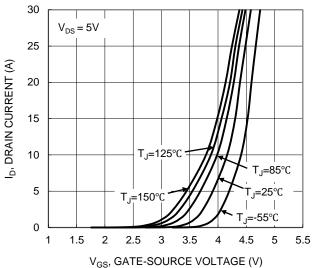
Figure 2. Typical Transfer Characteristic
