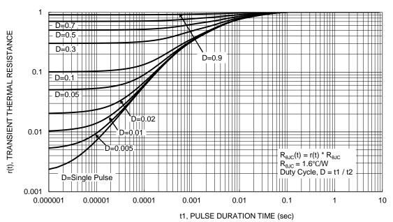
Figure 13. Transient Thermal Resistance
