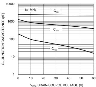
Figure 10. Typical Junction Capacitance
