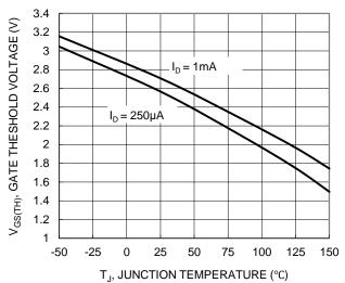
Figure 8. Gate Theshold Variation vs. Junction Temperature
