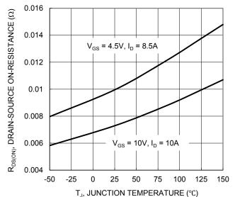
Figure 7. On-Resistance Variation with Junction Temperature
