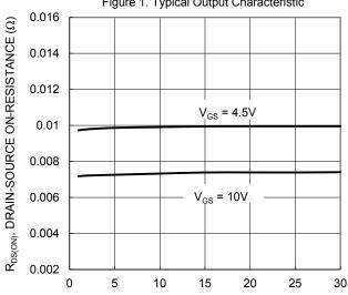
I<sub>D</sub>, DRAIN-SOURCE CURRENT (A) Figure 3. Typical On-Resistance vs. Drain Current and Gate Voltage
