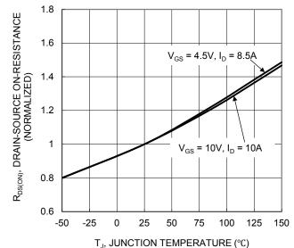
Figure 6.On-Resistance Variation with Junction Temperature
