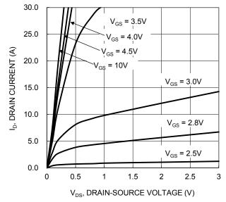
Figure 1. Typical Output Characteristic
