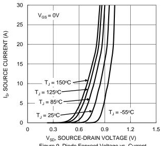
Figure 9. Diode Forward Voltage vs. Current
