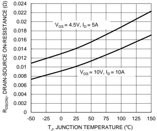
Figure 7. On-Resistance Variation with Junction Temperature
