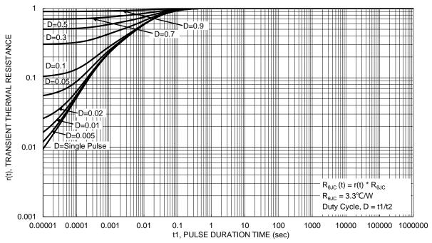
Figure 13. Transient Thermal Resistance
