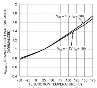
Figure 6. On-Resistance Variation with Temperature
