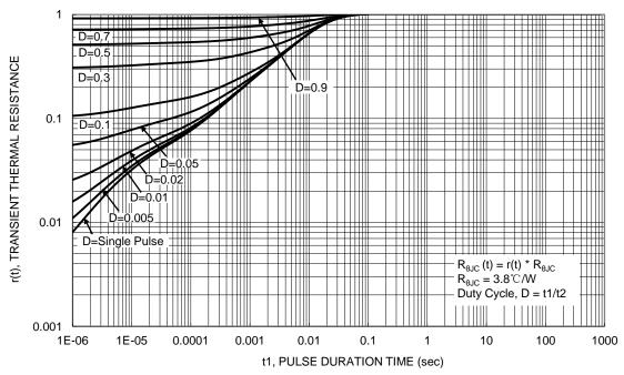
Figure 13. Transient Thermal Resistance
