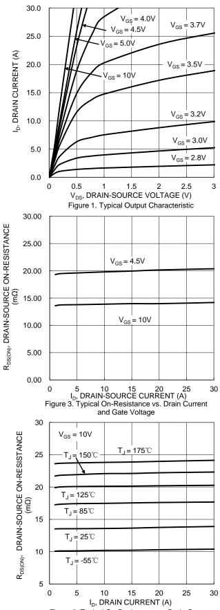
Figure 5. Typical On-Resistance vs. Drain Current and Temperature
