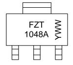
FZT1048A = Product Type Marking Code YWW = Date Code Marking Y or  $\overline{Y}$  = Last Digit of Year (ex: 8= 2018) WW or  $\overline{W}W$  = Week Code (01 to 53)
