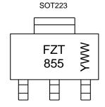
FZT 855 = Product Type Marking Code YWW = Date Code Marking Y or  $\overline{Y}$  = Last Digit of Year (ex: 7 = 2017) WW or  $\overline{W}W$  = Week Code (01–53)
