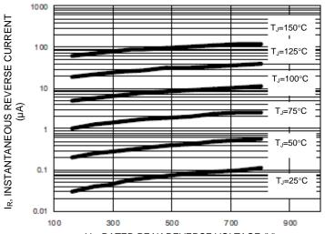
V<sub>R</sub>, RATED PEAK REVERSE VOLTAGE (V) Fig.5 Typical Reverse Characteristics
