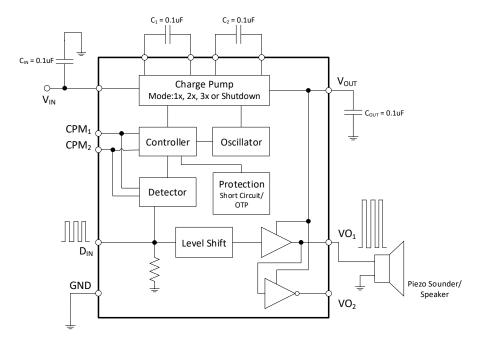
When using the PAM8904Q with a single ended output, the VO<sub>2</sub> pin should be left open circuit.
