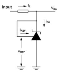
Figure 1. Test circuit for V<sub>KA</sub> = V<sub>REF</sub>
