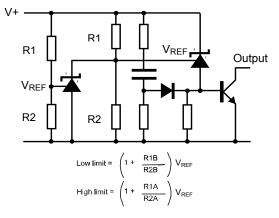
Over voltage / under voltage protection circuit
