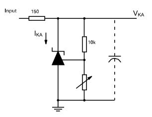
$V_{REF}$  <  $V_{KA}$  < 20V,  $I_{KA}$  = 10mA,  $T_{A}$  = +25°C Test Circuit for Stability Boundary Conditions
