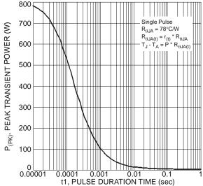
Figure 9 Single Pulse Maximum Power Dissipation
