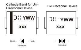
xx = Product Type Marking Code (See Electrical Characteristics Table) D!! = Manufacturers' Marking YWW = Date Code Marking Y = Last Digit of Year (ex: 1 for 2021) WW = Week Code (01 to 53)
