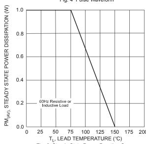
Fig. 6 Steady State Power Derating Curve
