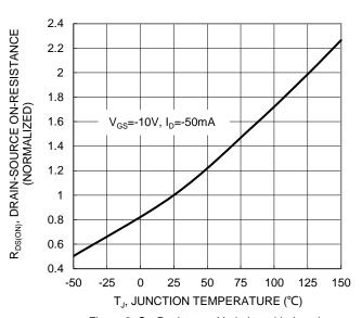
Figure 6. On-Resistance Variation with Junction Temperature
