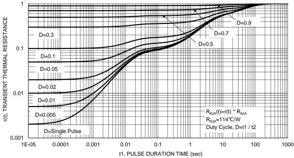
Figure 13. Transient Thermal Resistance
