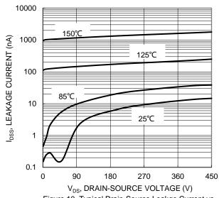
Figure 10. Typical Drain-Source Leakge Current vs Voltage
