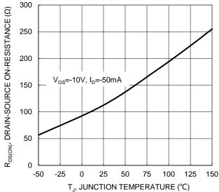
Figure 7. On-Resistance Variation with Junction Temperature
