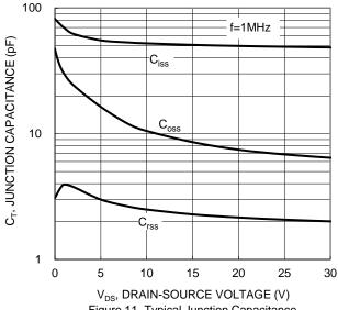
Figure 11. Typical Junction Capacitance
