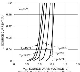
Figure 9. Diode Forward Voltage vs Current
