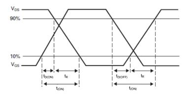
Switching time waveforms
