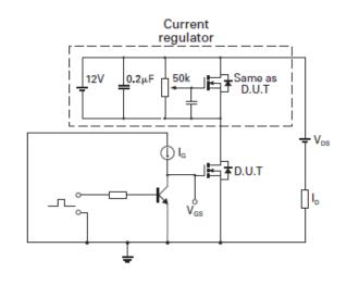
Gate charge test circuit
