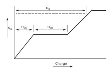
Basic gate charge waveform
