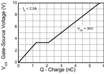
Gate-Source Voltage v Gate Charge
