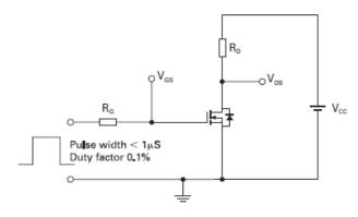
Switching time test circuit
