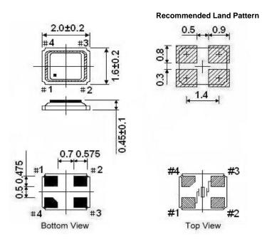
\*\* Recommended - Pin 1 & 3: CRYSTAL Pin 2 & 4: GND
