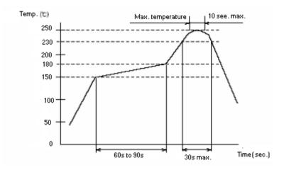
Notice 1.Soldering must be carried out without exceeding the allowable temperature and time as above chart.
