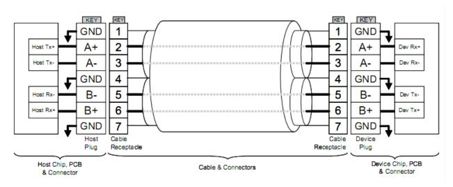
Figure 1-2 SATA Cable/Connector Connection Diagram
