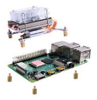
• Fixed Acrylic protection panel to Raspberry Pi with M2.5 screws.
