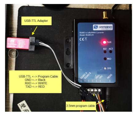
In PC, User needs to set **serial tool**(such as <u>putty</u>, SecureCRT) baud rate to **9600** to access to access serial console of RS485-LN. Below is the output for reference:
