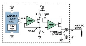
Figure 4. Discrete 4 mA to 20 mA implementation.
