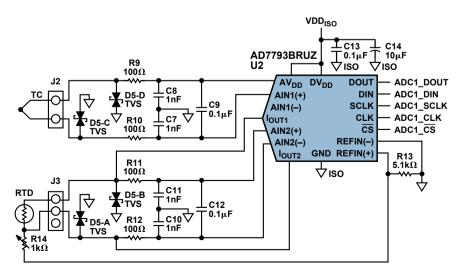
Figure 15. Analog input protection.
