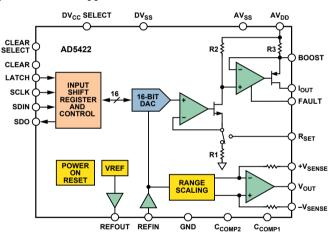
Figure 5. AD5422 programmable voltage/current output.
