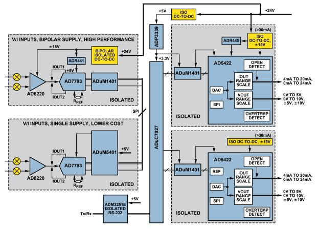
Figure 8. System-level design.
