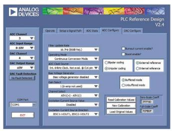
Figure 10. ADC Configure screen.
