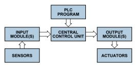
Figure 1. Typical top-level PLC system.
