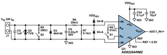
Figure 14. Analog input protection.
