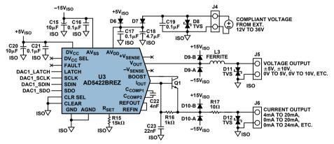
Figure 16. Analog output protection.
