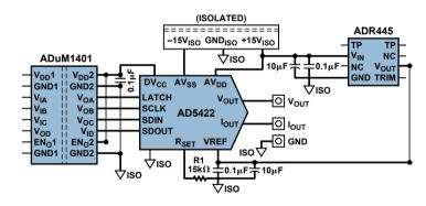
Figure 6. Output module block level.
