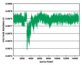
Figure 17. DAC channel dc voltage output. Radiated immunity 80 MHz to 1 GHz @ 10 V/mH.
