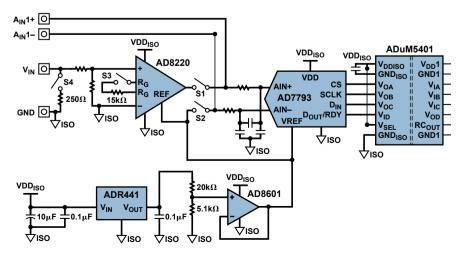
Figure 7. Input module design.
