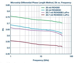
Figure 3. Dk and DF vs. frequency.1
