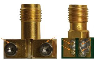
Figure 6. SMA with alignment features.
