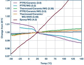
Figure 4. Dk change vs. temperature.1
