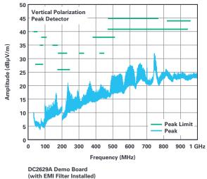
(with EIVII Fliter Installed) 3.3 V Input to 1.2 V Output at 7.5 A, f<sub>sw</sub> = 2 MHz
