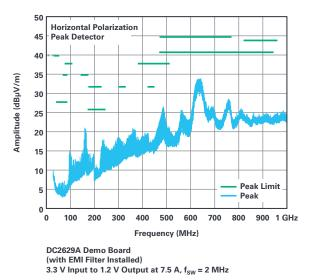
Figure 4. Radiated emissions for horizontal polarization.
