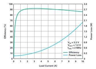
Figure 6. LTC3310S efficiency performance.
