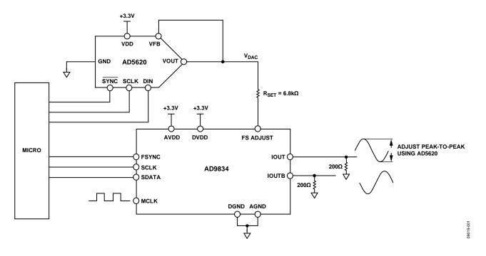
Figure 1. Low Power Amplitude Control Circuit for AD9834 DDS (Simplified Schematic: All Connections and Decoupling Not Shown)
