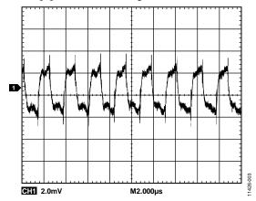
Figure 3. Output Voltage Ripple Before Low-Pass Filter
