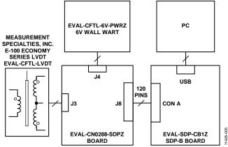
Figure 5. Test Setup Block Diagram
