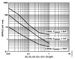
Figure 2. Output Voltage Ripple vs. Filter Capacitance
