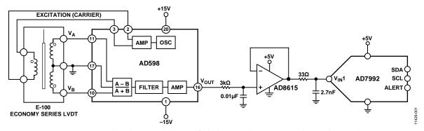
Figure 1. LVDT Signal Conditioning Circuit (Simplified Schematic: All Connections and Decoupling Not Shown)
