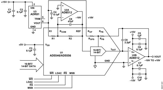
Figure 1. Bipolar Four-Quadrant Multiplying Mode with  $\pm 10$  V Output (Simplified Schematic)
