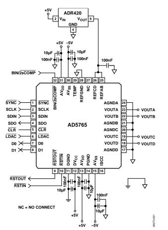
Figure 1. High Accuracy, Bipolar Configuration of the AD5765 DAC Using a Precision Reference
