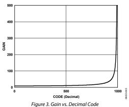
The maximum current allowed through the AD5292 is  $\pm 3$  mA, which limits the allowable circuit gain as a function of differential input voltage.
