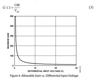
Equation 1 limits the maximum circuit gain to 500. Equation 2 can be solved for D, yielding Equation 4, which calculates the minimum allowable resistance (in terms of the digital code) in the AD5292 without exceeding the current limit.
