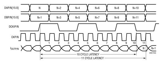
Figure 4b. Sample Waveforms - Dual-Port Operation
