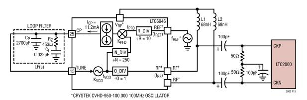
Figure 13. DAC Sample Clock Generation with the LTC6946
