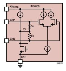
Figure 11. DAC Sample Clock Receiver
