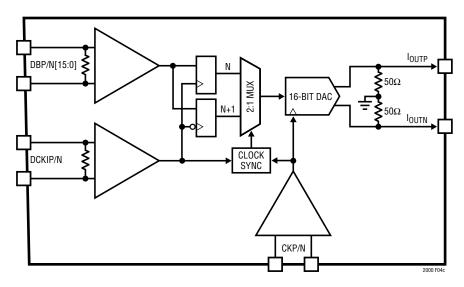
Figure 4c. Simplified Block Diagram – Single-Port Operation
