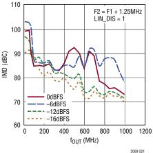
SFDR vs four and Linearization Setting, f<sub>DAC</sub> = 2.5Gsps
