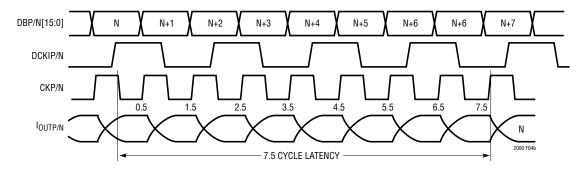
Figure 4d. Sample Waveforms - Single-Port Operation
