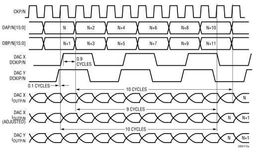
Figure 15a. Sample Waveforms — Synchronizing Multiple LTC2000s in Dual Port Mode
