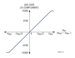
Figure 11. Fully-Differential Transfer Function
