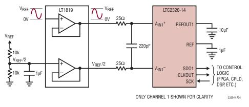
Figure 4. Pseudo-Differential Bipolar Application Circuit
