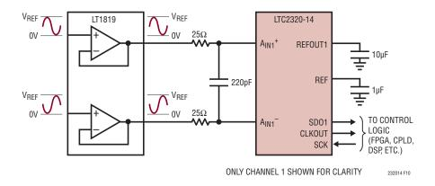
Figure 10. Fully-Differential Application Circuit
