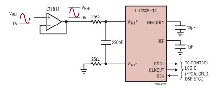
Figure 6. Pseudo-Differential Unipolar Application Circuit
