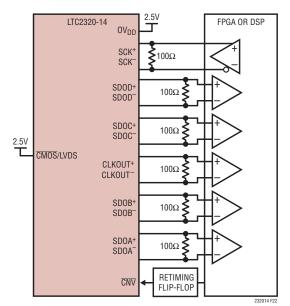
Figure 22. LTC2320-14 Using the LVDS Interface
