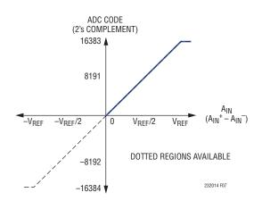
Figure 7. Pseudo-Differential Unipolar Transfer Function
