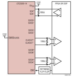
Figure 23. LTC2320-14 Using the LVDS Interface with One Lane 232014fa
