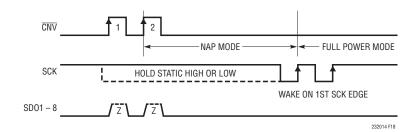
Figure 18. CMOS and LVDS Mode NAP and WAKE Using SCK
