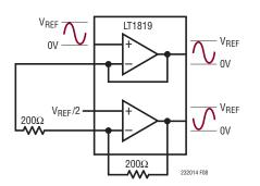
Figure 8. Single-Ended to Differential Driver
