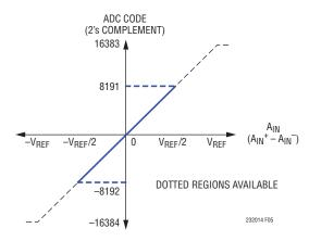
Figure 5. Pseudo-Differential Bipolar Transfer Function
