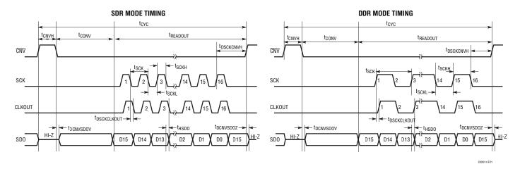
Figure 21. LTC2320-14 Timing Diagram
