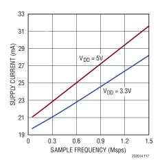
Figure 17. Power Supply Current of the LTC2320-14 Versus Sampling Rate
