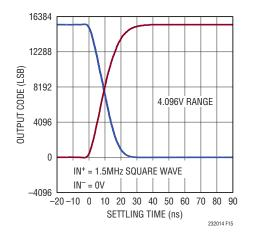
Figure 15. Transient Response of the LTC2320-14
