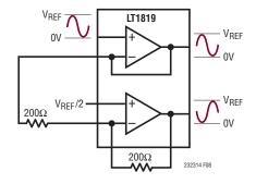
Figure 8. Single-Ended to Differential Driver
