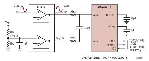
Figure 4. Pseudo-Differential Bipolar Application Circuit
