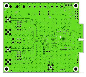
Figure 24. Layer 2, Ground Plane
