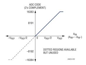
Figure 7. Pseudo-Differential Unipolar Transfer Function
