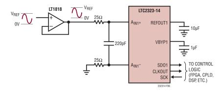
Figure 6. Pseudo-Differential Unipolar Application Circuit
