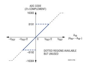
Figure 5. Pseudo-Differential Bipolar Transfer Function
