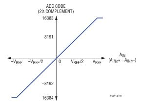
Figure 11. Fully-Differential Transfer Function
