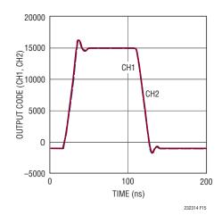
Figure 15. Transient Response of the LTC2323-14
