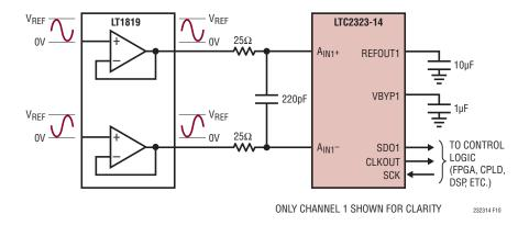
Figure 10. Fully-Differential Application Circuit
