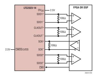
Figure 22. LTC2323 Using the LVDS Interface
