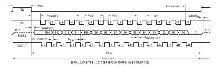
Figure 21. LTC2323-14 Timing Diagram
