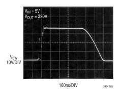
Figure 3. LT3484-0 SW Voltage Waveform
