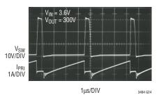
LT3484-0/LT3484-1/LT3484-2 Switch Breakdown Voltage
