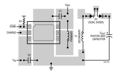
Figure 5. Suggested Layout: Keep Electrical Path Formed by C1, Transformer Primary and LT3484-0/LT3484-1/LT3484-2 Short
