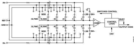
Figure 37. ADC Simplified Schematic
