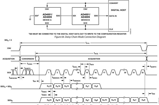
Figure 65. Daisy-Chain Mode Serial Interface Timing Diagram (Status Bits Not Shown)
