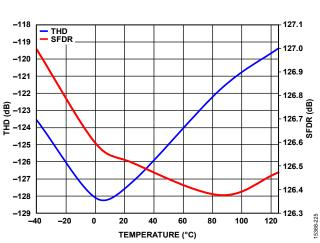
Figure 22. THD and SFDR vs. Temperature,  $f_{IN} = 1 \text{ kHz}$
