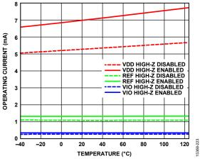
Figure 29. Operating Current vs. Temperature, AD4001, 2 MSPS
