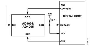
Figure 62. CS Mode, 4-Wire with Busy Indicator Connection Diagram
