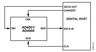
Figure 52. CS Mode, 3-Wire Turbo Mode Connection Diagram
