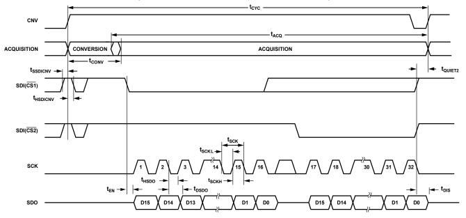
Figure 61. CS Mode, 4-Wire Without Busy Indicator Serial Interface Timing Diagram (Status Bits Not Shown)
