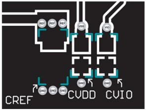
Figure 67. Example Layout of the AD4001 (Bottom Layer)
