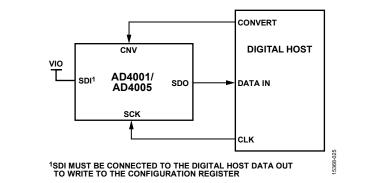
Figure 54. CS Mode, 3-Wire Without Busy Indicator Connection Diagram
