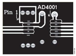
Figure 66. Example Layout of the AD4001 (Top Layer)
