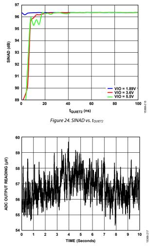
Figure 25. 1/f Noise for 0.1 Hz to 10 Hz Bandwidth, 50 kSPS, 2500 Samples Averaged per Reading
