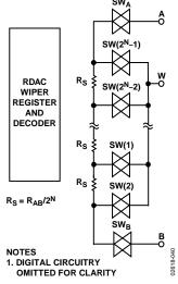
Figure 40. Equivalent RDAC Structure
