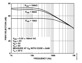
Figure 20. PSRR vs. Frequency
