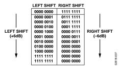
Figure 37. Detail Left and Right Shift Function
