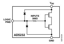
Figure 34. Equivalent ESD Digital Input Protection
