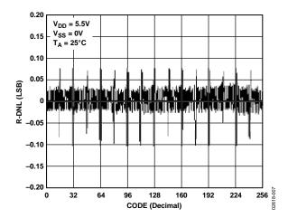
Figure 7. R-DNL vs. Code;  $R_{AB} = 10 \text{ k}\Omega$ , 50 k $\Omega$ , 100 k $\Omega$  Overlay
