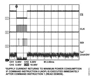
Figure 13. IDD vs. Time Read Mode
