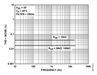
Figure 15. Total Harmonic Distortion + Noise vs. Frequency
