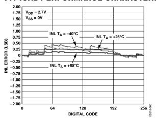
Figure 5. INL vs. Code;  $T_A = -40$ °C, +25°C, +85°C Overlay
