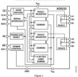
All internal register contents can be read via the serial data output (SDO). This includes the RDAC1 and RDAC2 registers, the corresponding nonvolatile EEMEM1 and EEMEM2 registers, and the 14 spare USER EEMEM registers that are available for constant storage.
