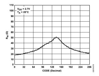
Figure 16. Wiper On Resistance vs. Code
