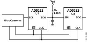
Figure 36. Daisy-Chain Configuration Using the SDO
