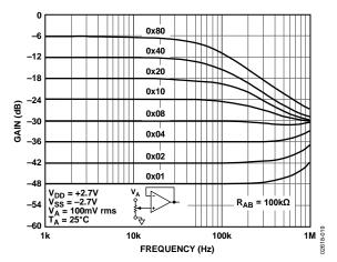
Figure 19. Gain vs. Frequency vs. Code,  $R_{AB} = 100 \, k\Omega$
