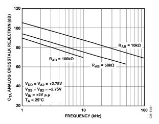
Figure 21. Analog Crosstalk vs. Frequency (See Figure 31)
