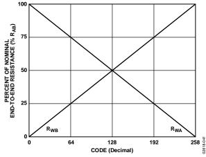
Figure 41. Symmetrical RDAC Operation
