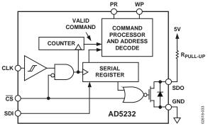
Figure 33. Equivalent Digital Input/Output Logic
