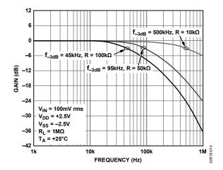
Figure 14. –3 dB Bandwidth vs. Resistance
