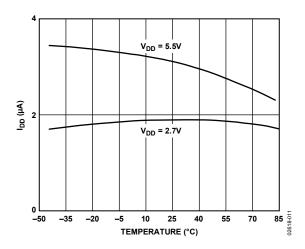
Figure 11. I<sub>DD</sub> vs. Temperature
