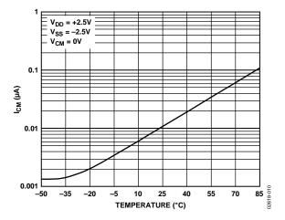
Figure 10. I<sub>CM</sub> vs. Temperature (See Figure 30)
