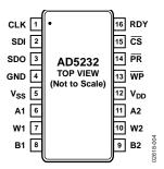
Figure 4. Pin Configuration
