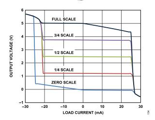
Figure 34. DAC Output Sink and Source Capability, Output Range = 0 V to 2 ×  $V_{REF}$
