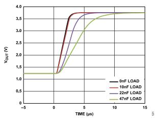
Figure 27. DAC Settling Time for Various Capacitive Loads
