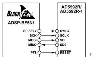
Figure 51. ADSP-BF531 SPI Interface
