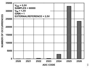
Figure 16. Histogram of ADC Codes,  $V_{DD}$  = 5.5 V
