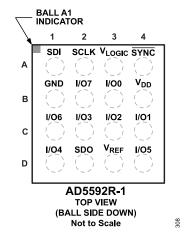
Figure 9. AD5592R-1 16-Lead LFCSP Pin Configuration
