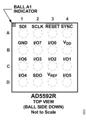
Figure 6. AD5592R 16-Ball WLCSP Pin Configuration
