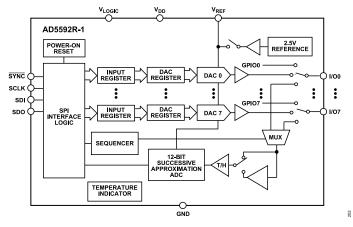
Figure 2. AD5592R-1 Functional Block Diagram
