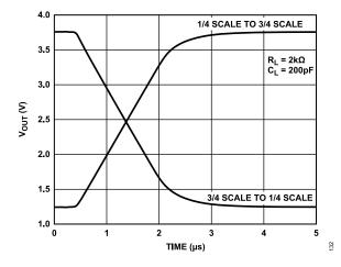
Figure 26. DAC Settling Time, Output Range = 0 V to 2 × V<sub>REF</sub>
