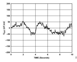
Figure 30. DAC 1/f Noise with External Reference
