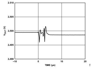
Figure 22. DAC Digital-to-Analog Glitch (Falling)
