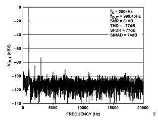
Figure 28. DAC Sine Wave Output, Output Range = 0 V to  $2 \times V_{REF}$ , Bandwidth = 0 Hz to 20 kHz
