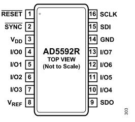
Figure 8. AD5592R 16-Lead TSSOP Pin Configuration
