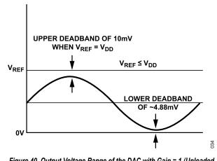
Figure 40. Output Voltage Range of the DAC with Gain = 1 (Unloaded Condition)
