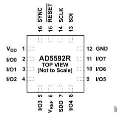
Figure 7. AD5592R 16-Lead LFCSP Pin Configuration
