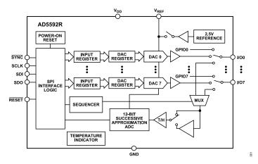
Figure 1. AD5592R Functional Block Diagram
