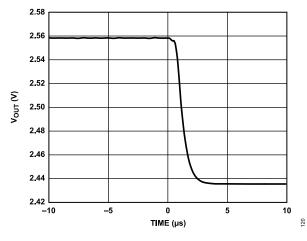
Figure 24. DAC Settling Time (100 Code Change, Falling Edge)
