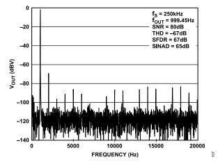
Figure 29. DAC Sine Wave Output, Output Range = 0 V to  $V_{REF}$ , Bandwidth = 0 Hz to 20 kHz
