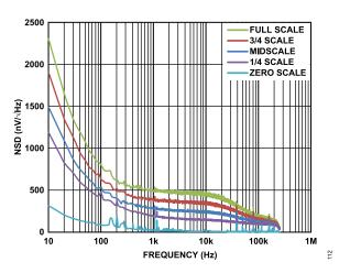
Figure 32. DAC Output Noise Spectral Density (NSD)
