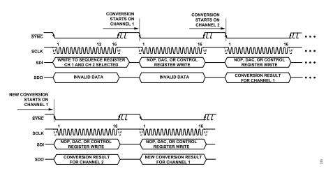
Figure 48. Multichannel, Repeating, ADC Conversion Sequence
