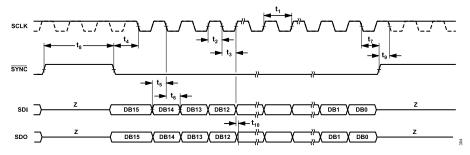
Figure 4. Serial Read and Write Timing Diagram
