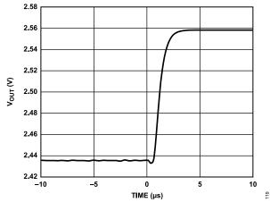
Figure 23. DAC Settling Time (100 Code Change, Rising Edge)
