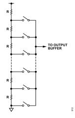
Figure 39. Simplified Resistor String Structure
