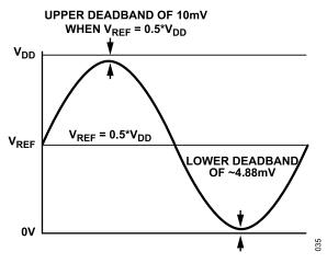
Figure 41. Output Voltage Range of the DAC with Gain = 2 (Unloaded Condition)
