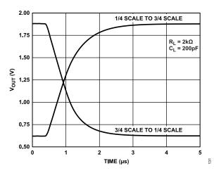
Figure 25. DAC Settling Time, Output Range = 0 V to V<sub>REF</sub>
