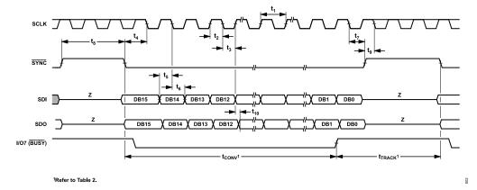
Figure 5. ADC Conversion Timing Diagram
