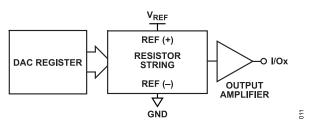
Figure 38. Internal Block Diagram of the DAC Architecture
