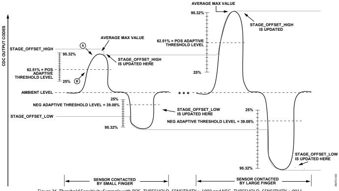
Figure 36. Threshold Sensitivity Example with POS\_THRESHOLD\_SENSITIVITY = 1000 and NEG\_THRESHOLD\_SENSITIVITY = 0011
