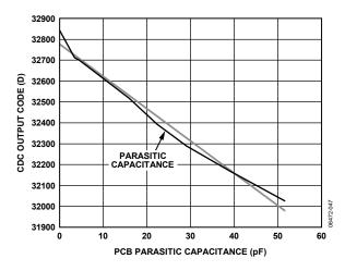
Figure 16. CDC Output Codes vs. Parasitic Capacitance
