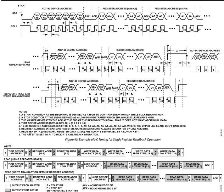
Figure 41. Example of Sequential I<sup>2</sup>C Write and Readback Operation
