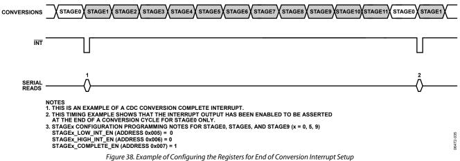
Figure 38. Example of Configuring the Registers for End of Conversion Interrupt Setup
