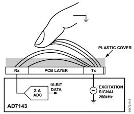
Figure 17. Single Layer Sensing Capacitance Method
