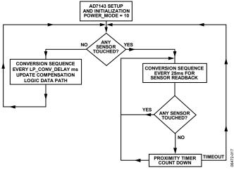
Figure 19. Low Power Mode Operation
