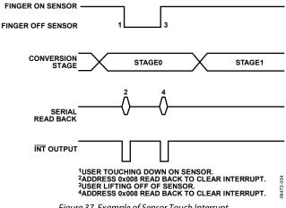
Figure 37. Example of Sensor Touch Interrupt
