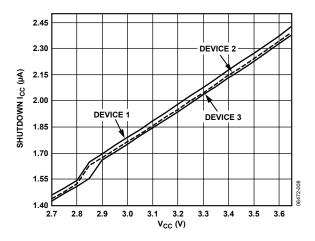
Figure 7. Shutdown Supply Current vs. Supply Voltage
