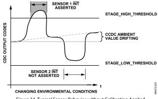
Figure 34. Typical Sensor Behavior without Calibration Applied
