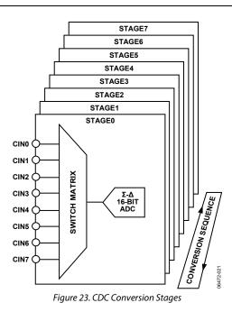
The number of required conversion stages depends completely on the number of sensors attached to the AD7143. Figure 24 shows how many conversion stages are required for each sensor, and how many inputs each sensor requires to the AD7143.
