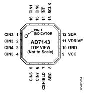
Figure 3. Pin Configuration
