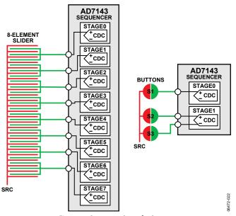
Figure 24. Sequencer Setup for Sensors
