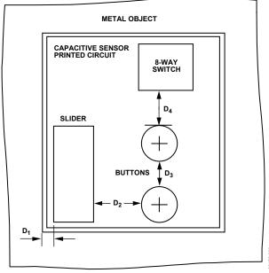
Figure 42. Capacitive Sensor Board Mechanicals Top View
