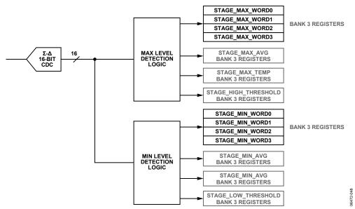
Figure 32. AD7143 Maximum and Minimum Level Detection Logic
